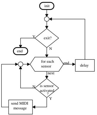
Figure 3: Fluxogram of the software running on the PC.
