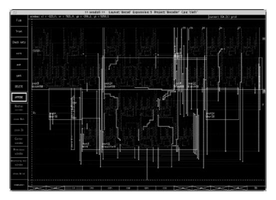
Figure 5: Layout of the decoder integrated circuit designed for the system.
