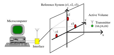
Figure 4: Position acquisition system.
