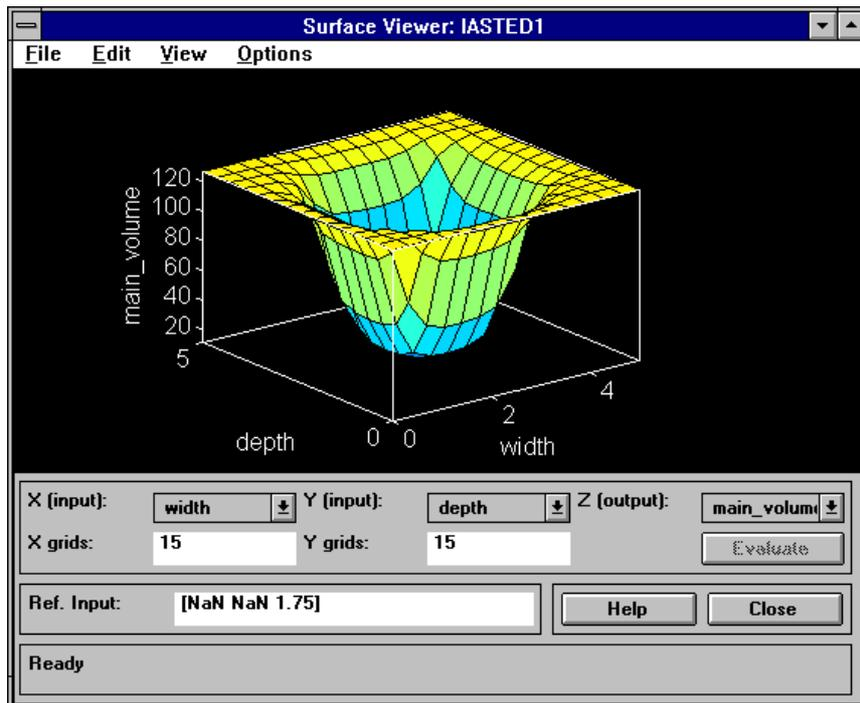
Figure 6: Fuzzy control of volume based on mapping the dancer position.
