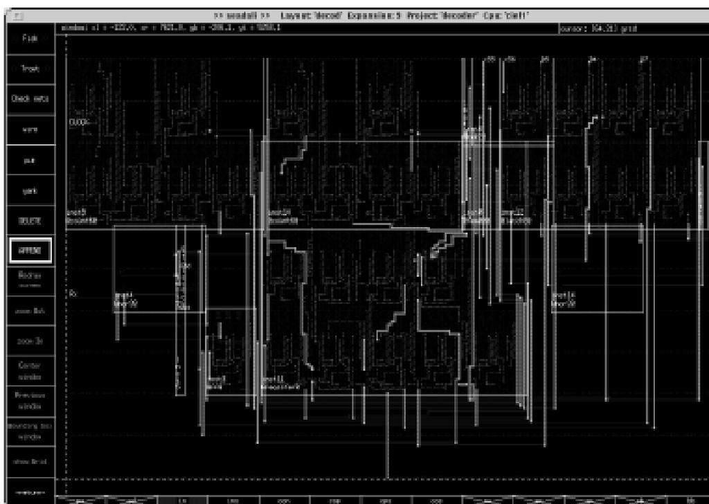
Figure 5: Layout of the decoder integrated circuit designed for the system.
