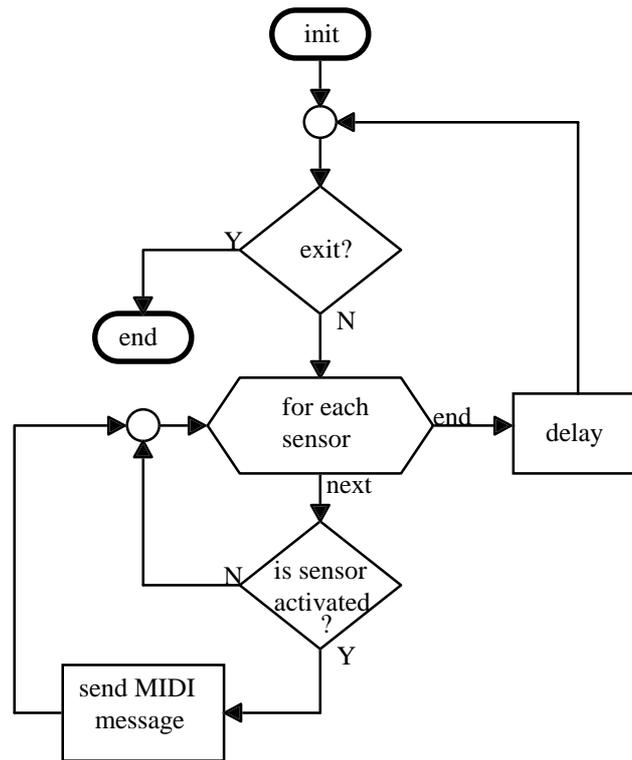
Figure 3: Fluxogram of the software running on the PC.
