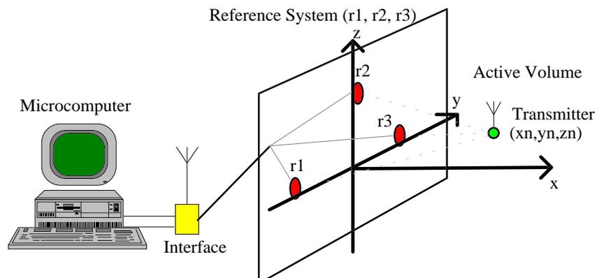
Figure 4: Position acquisition system.
