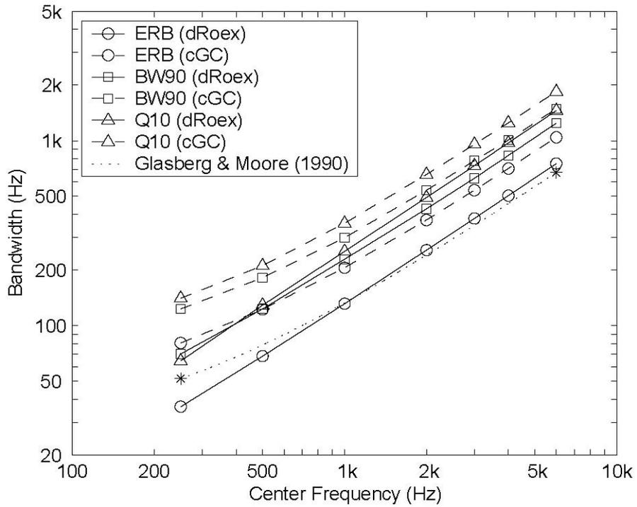
**Fig. A1.** Comparison of three bandwidth measures for the compressive gammachirp (cGC) filter and double roex (dRoex) filter when the level is 50 dB SPL.
