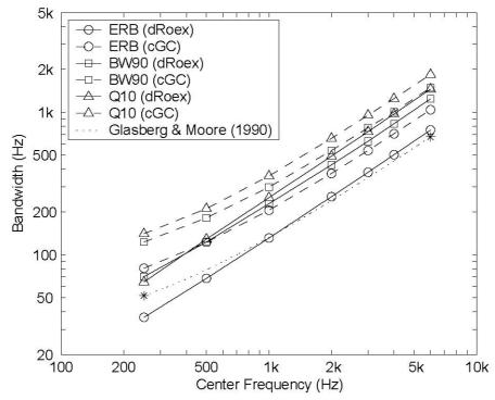
**Fig. A1.** Comparison of three bandwidth measures for the compressive gammachirp (cGC) filter and double roex (dRoex) filter when the level is 50 dB SPL.
