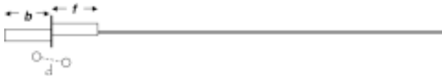
Figure 7. Parameters in the algorithm: the forward and backward window sizes, f and b .
