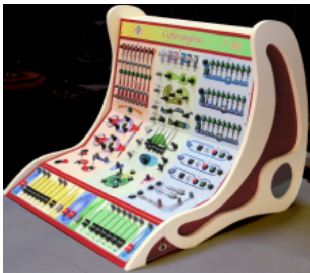
Figure 2. Frontview of the main surface control and mixing desk.
