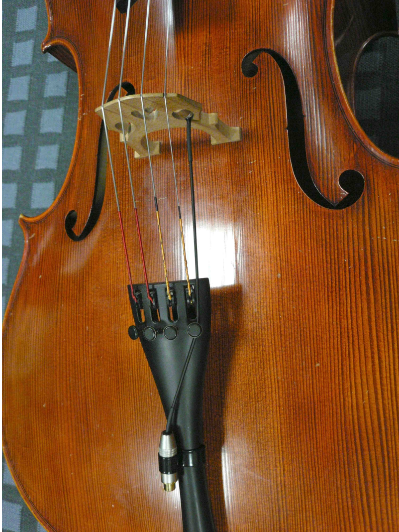
Figure 8: A Stat-C system on a cello
