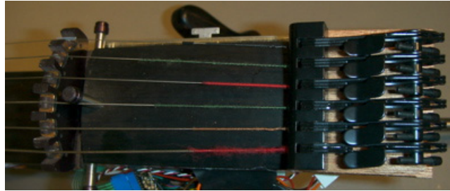
(a) Cello heel with string tuning device
