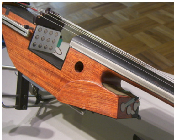
(c) Cello body showing neck and body FSR
