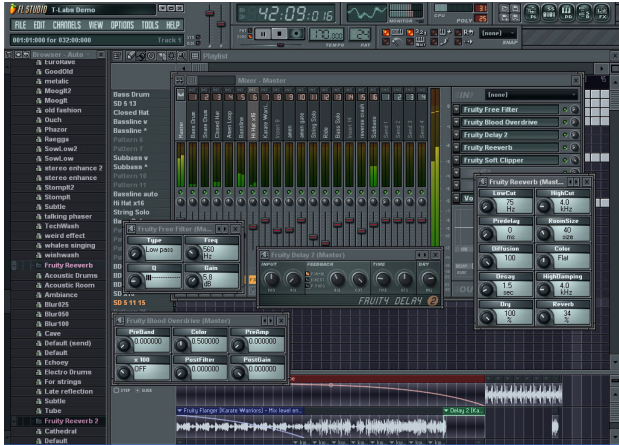
Figure 7: An example mapping of CaMus to the commercial sequencing software FruityLoops (by Image-Line Software). Various parameters are mapped to the knobs of various effects boxes via MIDI.
