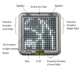
Figure 2. Interface of TENORI-ON (Surface)
