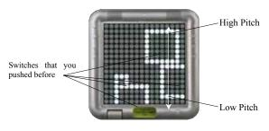
Figure 5. Real Time Rec Mode
