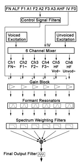
Figure 4: Block diagram of speech synthesizer
