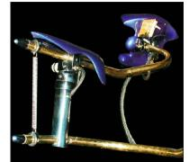
Figure 2: Static force feedback - springs & adjustable friction
