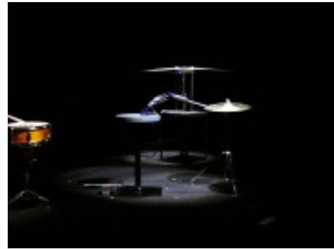
Fig.4: Pipe Robot appears behind the Cymbal Robot on this photo. Pipe robot changes the pitches according to the speed of spins.
