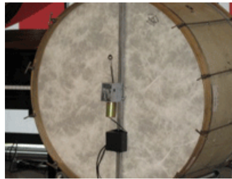
Fig. 3—Bass drum with BeaterBot.
