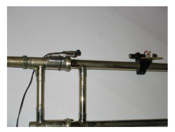
Figure 3. Slide with the position sensors
