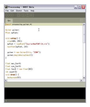
Figure 7: An example of a 'sketch.' Since all I/O module functions are represented as methods of the 'Gainer' class, a user doesn't have to deal low messages from/to an I/O module.
