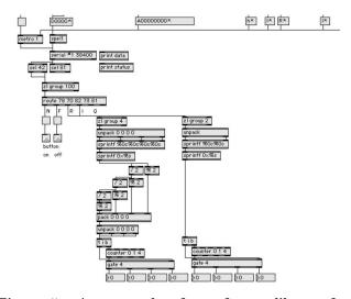
Figure 5: An example of a software library for Max/MSP. The library encapsulates low messages between a PC and an I/O board, representing them as higher level messages.
