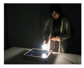
Figure 13: Input is brightness information from CdS sensors. Output is lights from white LEDs and corresponding sounds from a PC.
