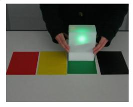
Figure 11: Input is color information from a RGB color sensor. Output is a light from a RGB color LED and corresponding sounds from a PC.
