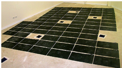
Figures 2. & 3. The Sensate Lab (2 views) showing the "invisible" pressure sensitive floor mats, triggering the visual and auditory sound system and (bottom) before carpeting, networked to the Teleo (analog to digital in/out) modules for conversion to a USB interface [20].
