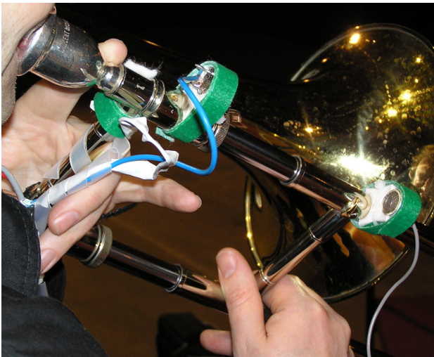
Figure 1. The uSlide transmitter (right of photo) and receiver (upper middle). The player's left forefinger is resting on the mouthpiece, next to the Trombone push-button (hidden). The nylon coil-wrap (centre left) is an easily released tether for the umbilical cable.
