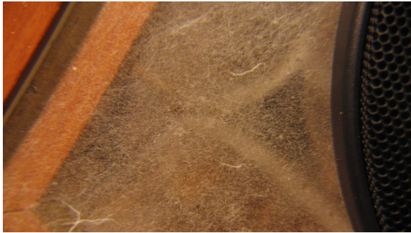
Fig. 3. Construction: close up of bleached mulberry fibres which enhance light absorption properties of the surface
