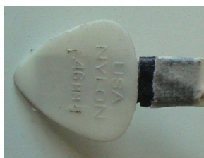
Figure 4. The plectrum-like controller: the sensor is between two glued thin plectras (0.46 mm)
