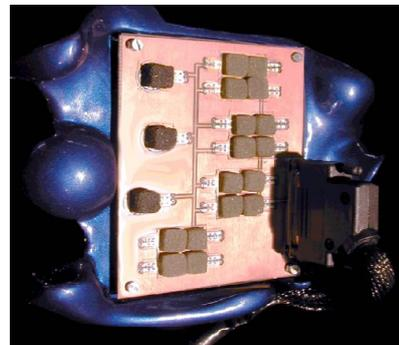
Figure 1: The hand of MI3 with soft keys
