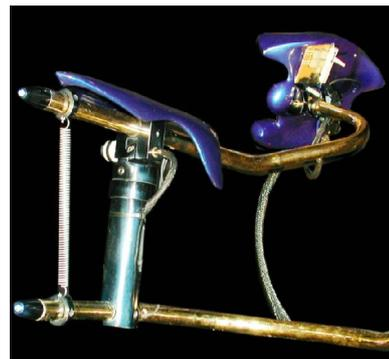
Figure 2: Static force feedback - springs & adjustable friction
