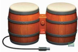
Figure 3: Shown above is the congo drum interface for Nintendo's Donkey Konga . It is the closest match to an real musical instrument gaming interface, as the device produces acoustic sound in addition triggering electronic events. The musical input is simple momentary controls in the form of beats, the game accepts no harmonic or melodic input.
