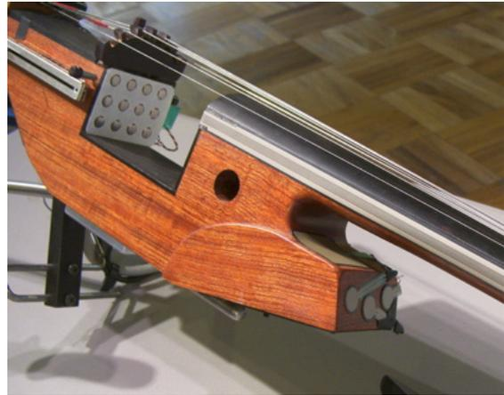
Figure 2. Cello Body showing neck and body FSR
