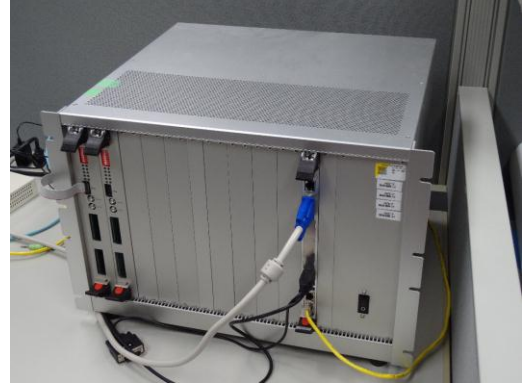
Figure 2: Photograph of the hardware accelerator using FPGAs.
