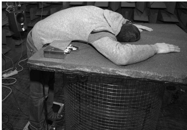
Figure 2: Subject position during the measurements. On top left, the boom-controlled loudspeaker used for sweep reproduction.
