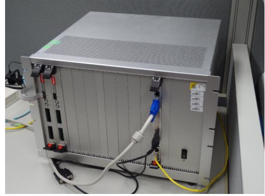
Figure 2: Photograph of the hardware accelerator using FPGAs.
