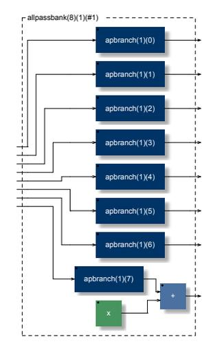
Figure 7: Nonlinear allpass bank showing mesh corner excitation. This is an expansion of the block labeled “apbank (8) (#1)” in Fig. 6.
