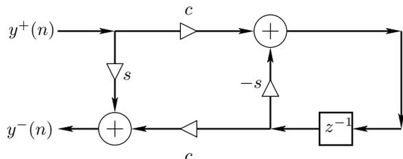
Figure 2: First-order normalized ladder allpass filter, with coefficients  $c = \cos(\theta)$  and  $s = \sin(\theta)$ ,  $\theta \in [-\pi, \pi]$ .
